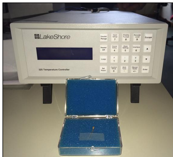
Figure 8: LakeShore temperature measurement system. On the blue box is visible the calibrated temperature sensor.
